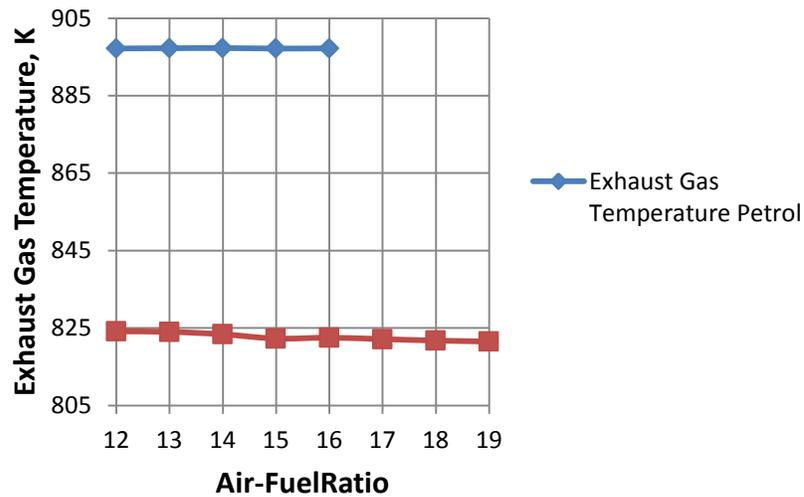
**Fig.8 Effect of Air-Fuel Ratio on Exhaust Gas Temperature.**
