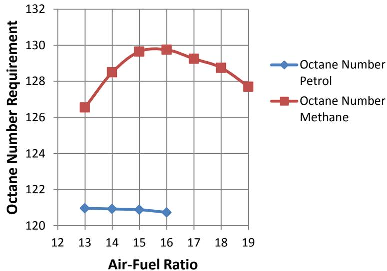
**Fig.1 Effect of Air-Fuel Ratio on Octane Number Requirement**
