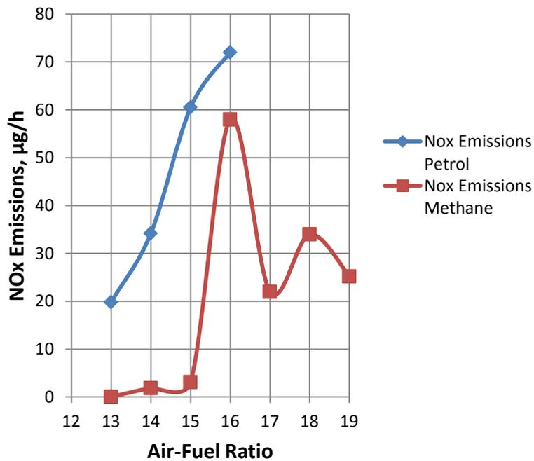
**Fig.7 Effect of Air-Fuel Ratio on NOx Emissions.**
