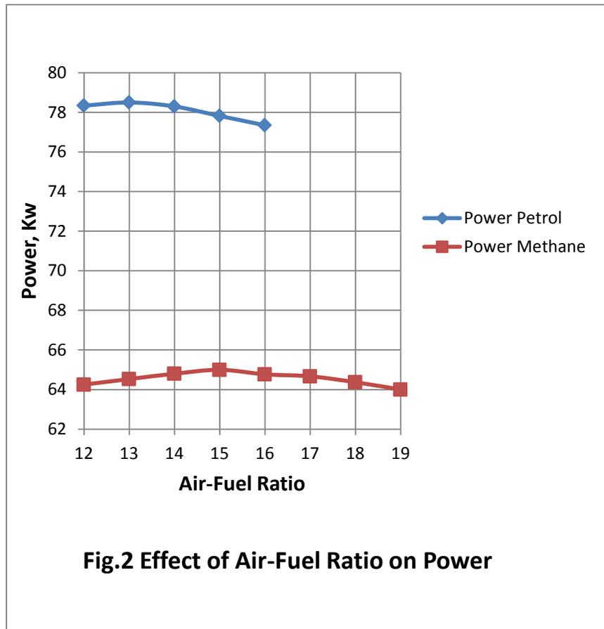
**Fig.2 Effect of Air-Fuel Ratio on Power**
