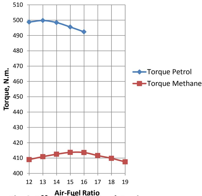
**Fig.3 Effect of Air-Fuel Ratio on Torque**
