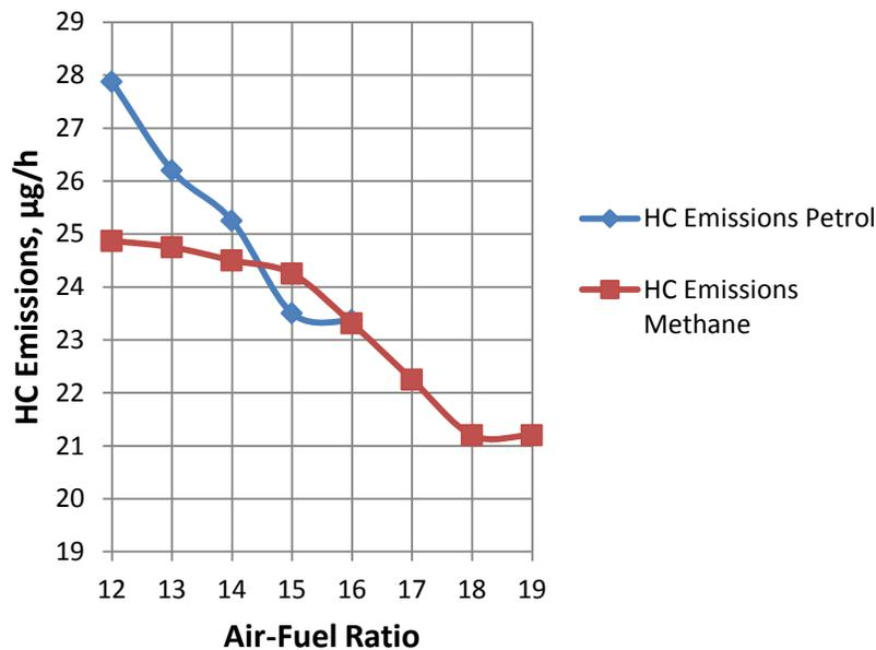
**Fig.6 Effect of Air-Fuel Ratio on HC Emissions**
