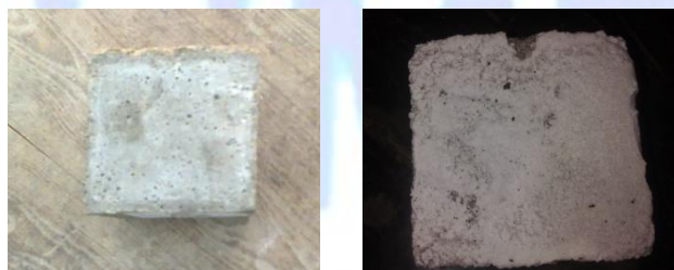
Figure 7: Photographs of corroded specimen surface taken after four weeks of exposure in 10% solution of nitric Acid
