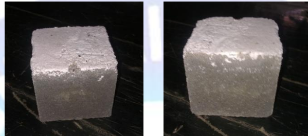
Figure 6: Photographs of corroded specimen surface taken after four weeks of exposure in 10% solution of H_2SO_4
