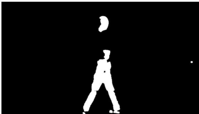
Figure 2: Human silhouette obtained by background subtraction
