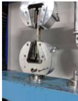
Fig 5 Testing of scarf adhesive joint on UTM
