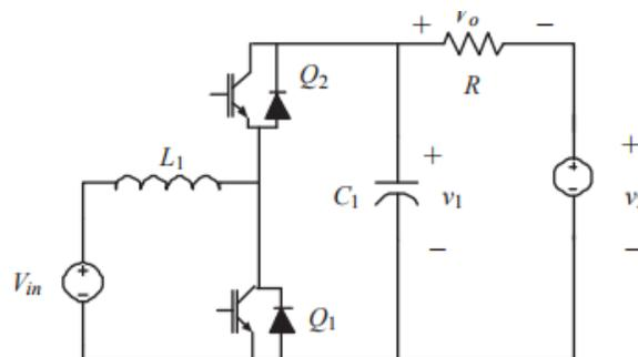
**Fig. 3** Boost inverter model with replacement of a voltage source
