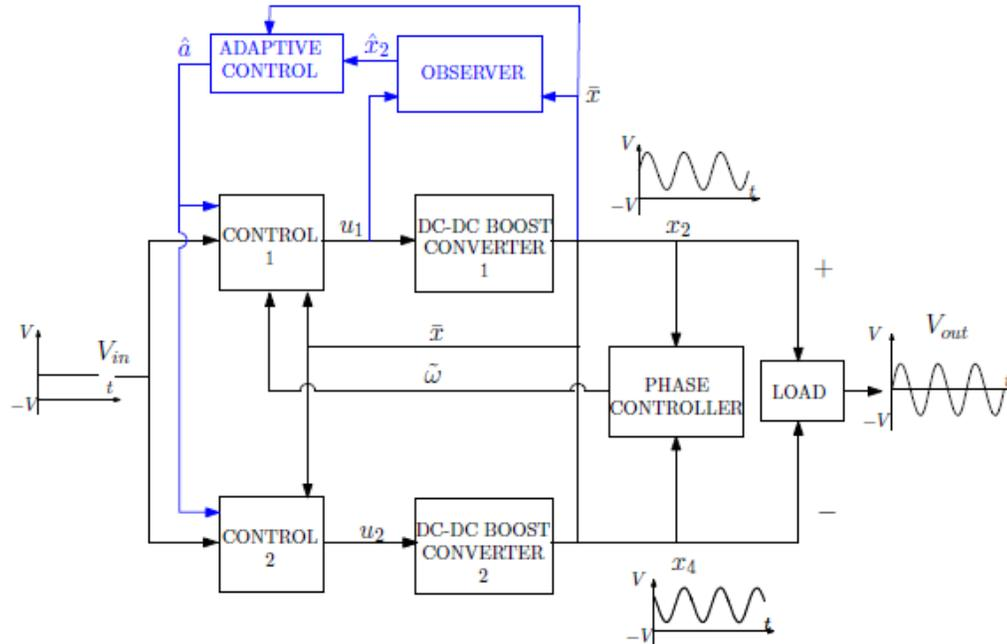
Fig. 4 Controlled boost inverter with observer
