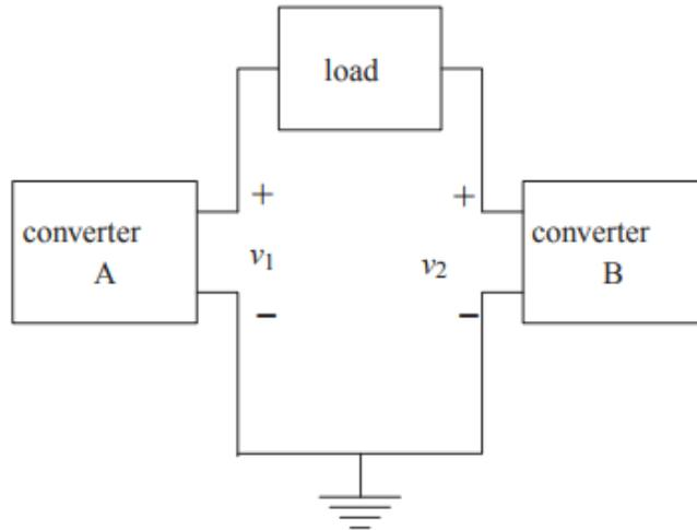
**Fig. 1**Basic representation of the boost inverter
