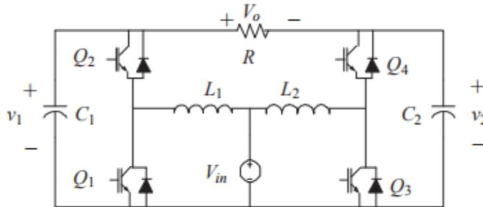
**Fig.2**Boost inverter model
