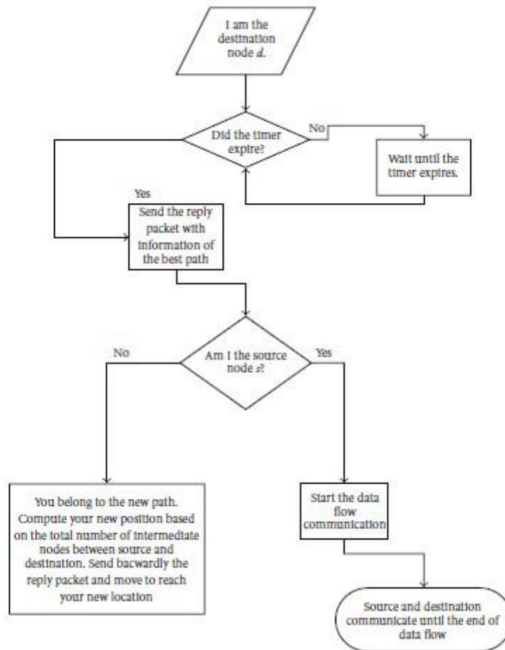
**Figure: 3 Reply Phase of RCPM**
