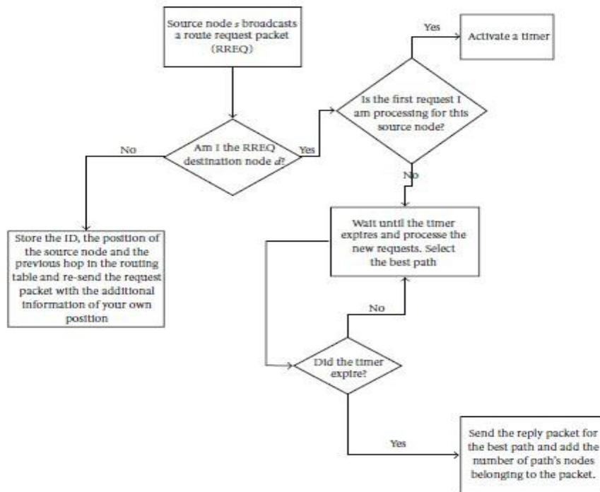
**Figure: 2 Routing Request Phase of RCPM**
