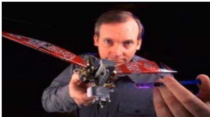
An "electromechanical multimode" micro UAV is being developed by Robert Michelson and his design team at the Georgia Tech Research Institute
