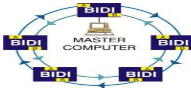
Figure 6: Dual Counter-rotating Ring Topology
