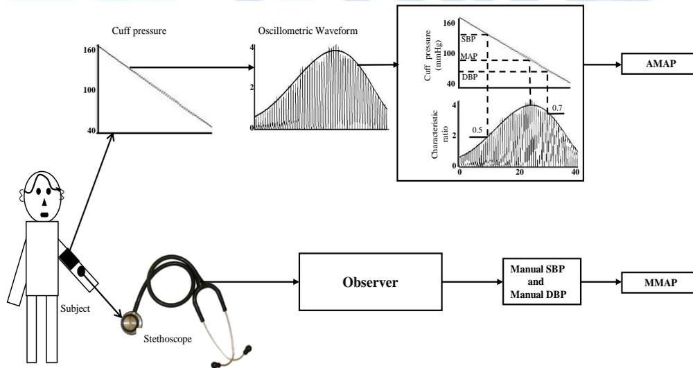
Figure 1: Schematic representation of BP measurement on a subject.
