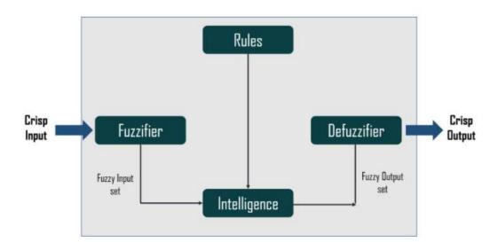
**Fuzzification** – This step converts inputs or the crisp numbers into fuzzy sets. You can measure the crisp inputs by sensors and pass them into the **control system** for further processing.
