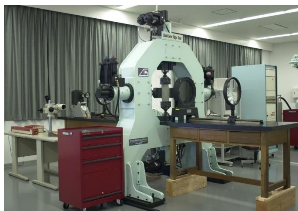
Figure 2. Photoelastic experiment system with biaxial loading device
