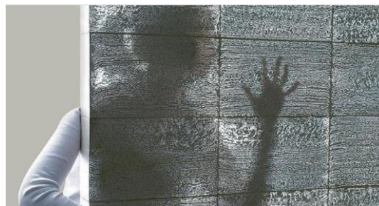
Figure 4 Translucent (Transparent) concrete [13]
