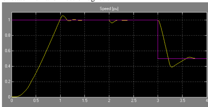
Figure4. Motor speed and reference speed during using HPSO
