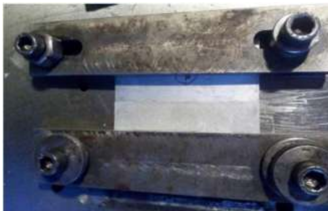
Figure 2 Test plated clamped to the backing plate during friction stir welding process
