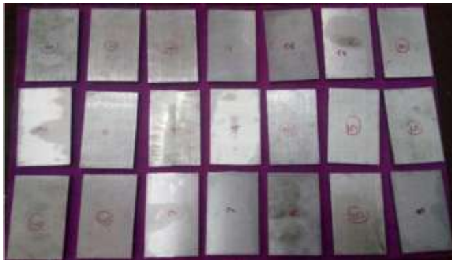
Figure 1 Plates prepared for friction stir welding from stir casting (100 mm X 50 mm X 6 mm size)
