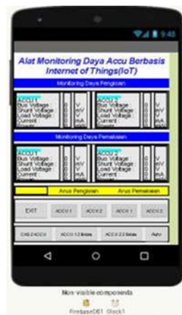
Figure 14. Accu Power Monitoring Interface Design
