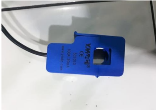
Figure 1. Current sensor STC013-030
