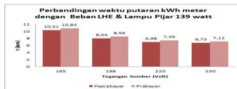
Figure 4.2 Comparison of prepaid and postpaid kwh meter rotation using LHE load The graph above shows the rotation of the kwh meter with a voltage of 165 volts, there is a difference between postpaid and prepaid, while at normal voltage of 220 volts there is also a difference between the two.
