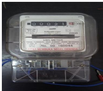
Figure 2.1 Kwh Meter Postpaid.
