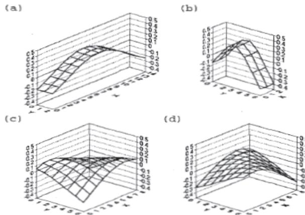
**Figure 3.2 Character extraction filters (a) Vertical. (b) Horizontal. (c) Left diagonal. (d) Right diagonal [8].**
