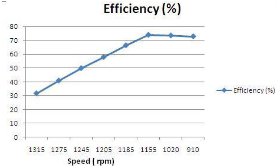
Graph: 5.3 Efficiency Vs Speed for Conventional Flywheel.
