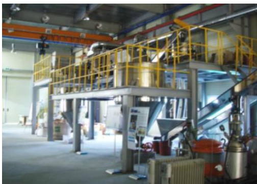
Fig.6.200 kg/hour MSWI bottom ash multi-process Fig.7. 20 tons/hour Removal process model of heavy metals chlorides from MSWI bottom ash
