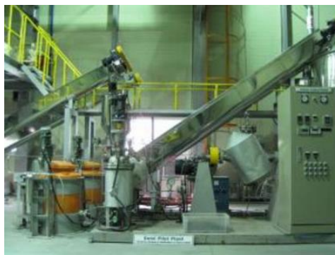
Fig.6.200 kg/hour MSWI bottom ash multi-process Fig.7. 20 tons/hour Removal process model of heavy metals chlorides from MSWI bottom ash
