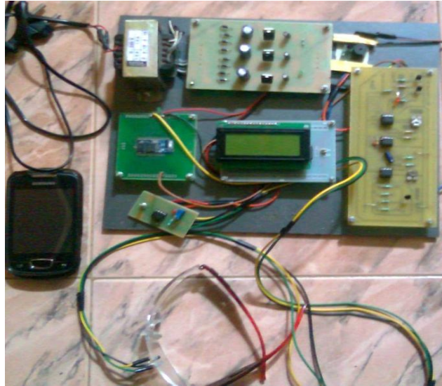
Fig 5: Hardware kit for driver fatigue level monitoring
