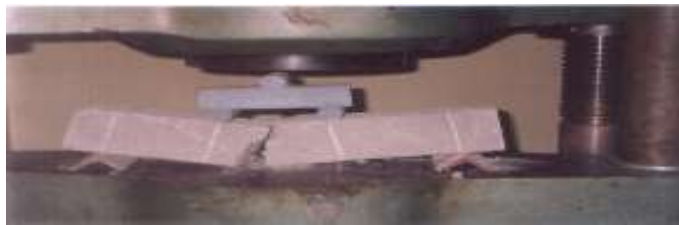
Fig: 9 TYPICAL FRACTURE PATTERN OF BEAM SPECIMENS DUE TO FLEXURAL LOAD (M20, 0% Fly ash)
