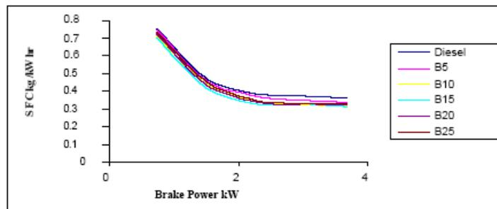
Fig.3 Comparison of BSFC v/s Brake power
