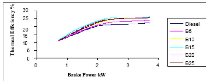
Fig.1 Thermal efficiency v/s Brake power
