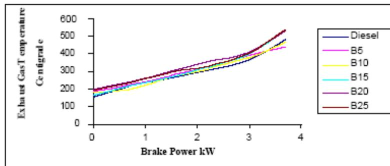
*Fig.5 Exhaust Gas Temperature v/s Brake power*
