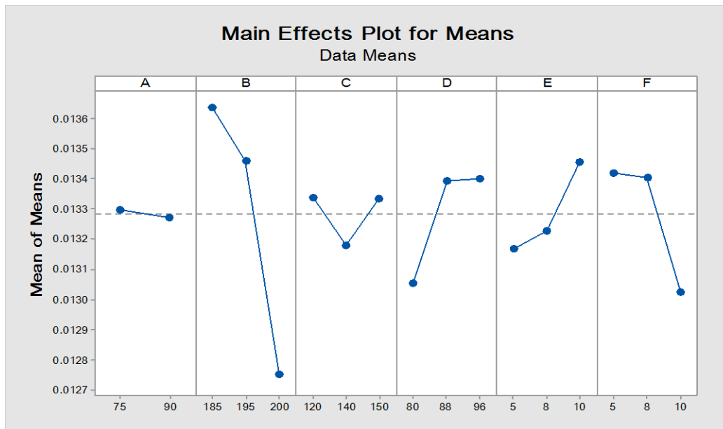
Figure 5: Average response mean of means for factors graph for mold shrinkage
