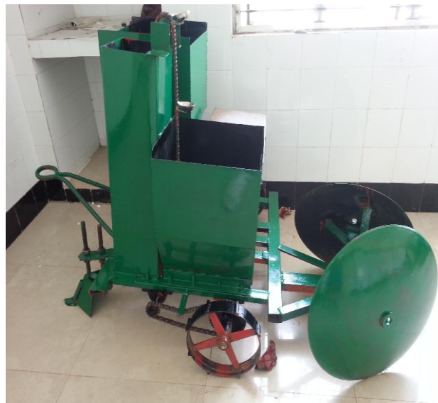
Fig. 18 Potato Planting Machine
