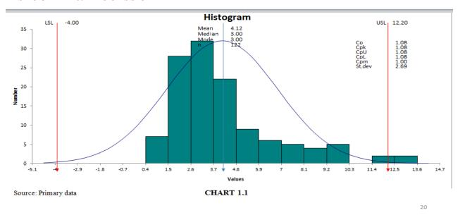
The above histogram chart shows that the normal frequency distribution of collected data. Cp = 1.08 which means Cp> 1 that the process variation is less than the specification (i.e.) the process is capable of meeting the specifications.
