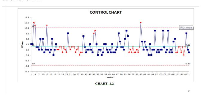
The above control chart shows that the subgroup of 32 were not within the control limits and it was found to be out of control among other sub groups. The above control chart shows the points that are closer and above the upper control limit (UCL) which is treated as special cases.
