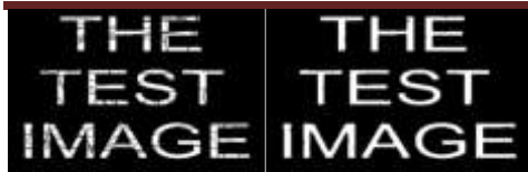
Fig.7: Closing: The original image dilated and then eroded. Most holes are filled. Morphological Opening and closing
