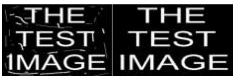
Fig. 6: Opening: The original image eroded and dilated twice(opened) Most noise is removed
