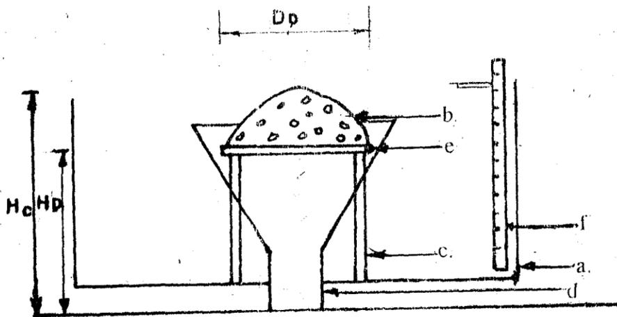
Fig.3-4: Apparatus for determination of static angle of repose .
