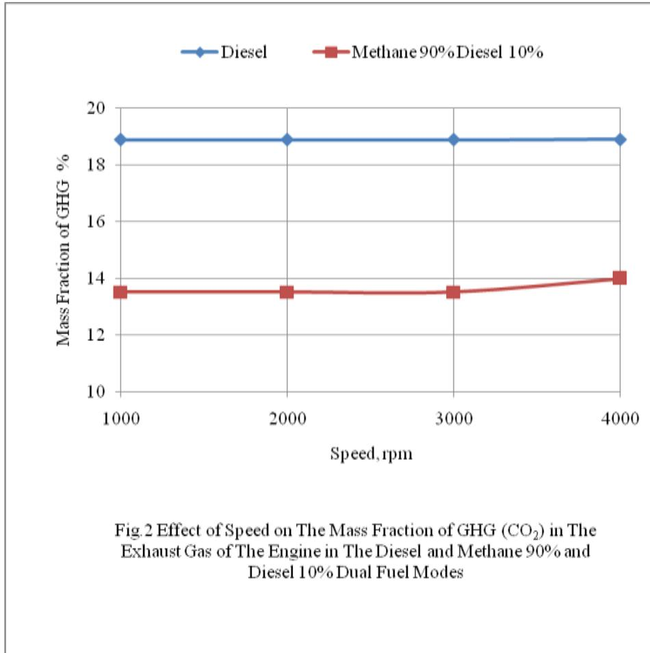
Fig.2 Effect of Speed on The Mass Fraction of GHG (CO<sub>2</sub>) in The Exhaust Gas of The Engine in The Diesel and Methane 90% and Diesel 10% Dual Fuel Modes
